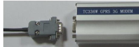
Figure II.2: Modem Communication Port
