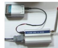
Figure III.2: Modem Connected to POE
